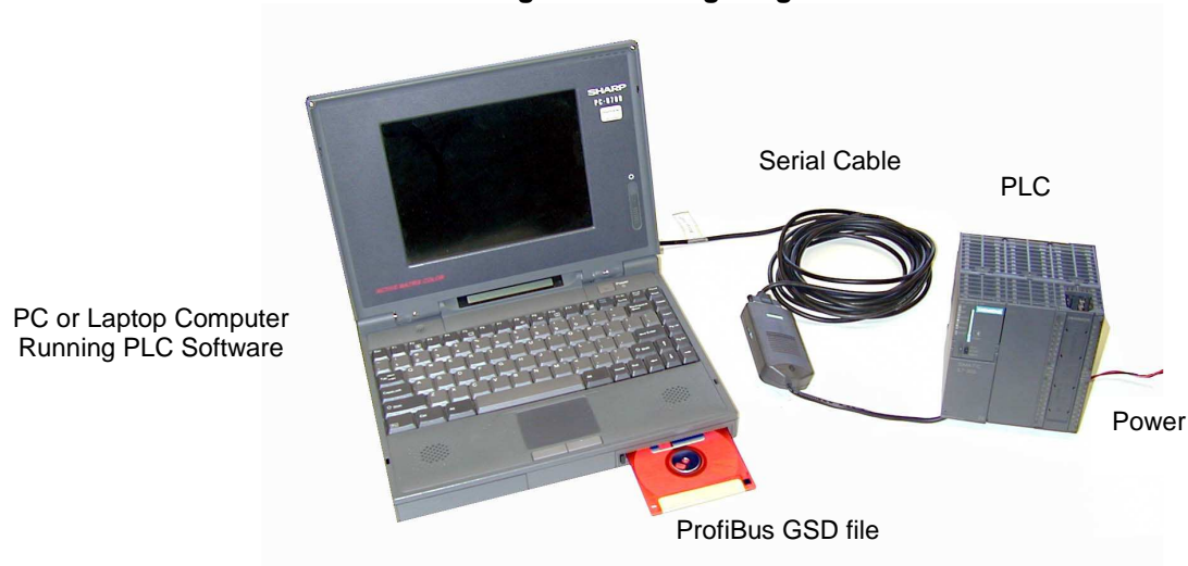
Figure 2 Configuring the PLC
