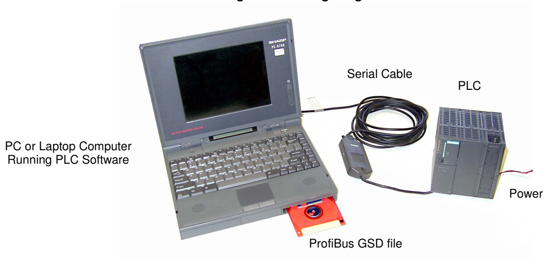
Figure 2 Configuring the PLC
