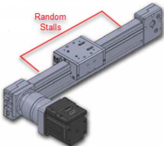
Figure 1: Random stalls area along the actuator length
