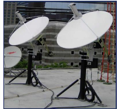
**Big** plans are in M<sup>2</sup>'s future with the help of the SmartMotor, including a cost-effective means of "auto-tracking." Auto-tracking is accomplished by writing code into the controller unit specifying a certain object's trajectory, while a separate antenna module with receiver is set up to judge signal strength of the object in orbit and automatically adjust the equations in the system to correct the slightest position error and therefore receive the strongest signal data.
