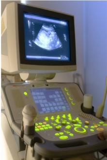
Ultrasound transducers are the wands that send and receive the sound waves, converting the electrical potential energy into mechanical sound wave vibrations and vice versa. The transducer is the mouth and ears of the ultrasound machine, reading the ultrasound waves through tiny crystals in the end of the transducer which vibrate when voltage is applied to them (the piezoelectric effect). Since many different structures and materials can
