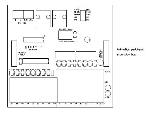
The jumpers on the DINIO-RS485 are intended primarily to allow the user to connect the RS-485 connections, +5V power and ground to the expansion bus.
