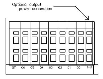
The two-stack output terminal labeled PWR allows you to power the inputs and outputs separately by removing the jumper adjacent to the PWR two stack terminal. That is, the jumper connects the +24V of the input and output sections of the DINIO-RS485. If you remove the jumper, you must power the output section of the unit at the two stack PWR terminal block - it will not operate without it.
