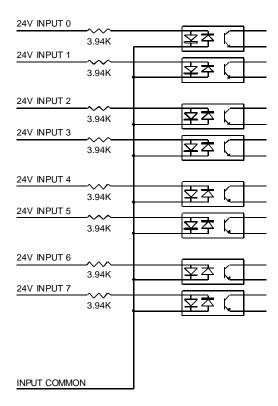
By default, the input +24V is connected to the output +24V. The power voltages of the input and output stages can be separated by removing the jumper adjacent to the PWR two stack terminal block. In any case, the user must provide +24V power to the input terminal block in order for the DINIO-RS485 unit to function.
