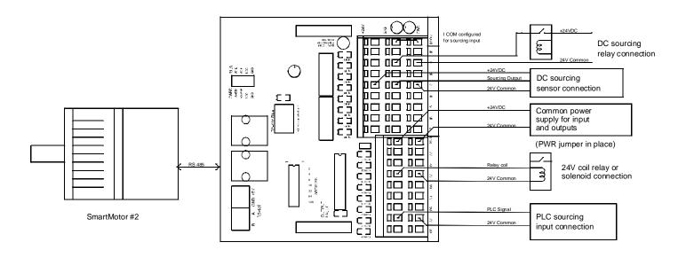
In general, the SmartMotor™ communicates with the DINIO-RS485 through its channel 1 serial port. On the SmartMotor™, the serial port is initialized through the OCHN command. Commands are then issued from the SmartMotor™ to the DINIO-RS485 to read the I/O states and set or reset the outputs.
