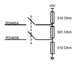
Due to the nature of RS-485, the biasing resistors, or their equivalent, must exist somewhere in a RS-485 communication bus. The terminator is required in particularly noisy environments or high baud rates. If these resistors are absent, intermittent or continuous communication errors may result. In many cases, RS-485 transceivers that are designed as masters, or hosts, already incorporate this biasing, but not the terminating resistor.
