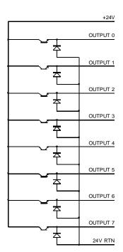
If you remove the jumper, you must power the output section of the unit at the two stack PWR terminal block - it will not operate without it.
