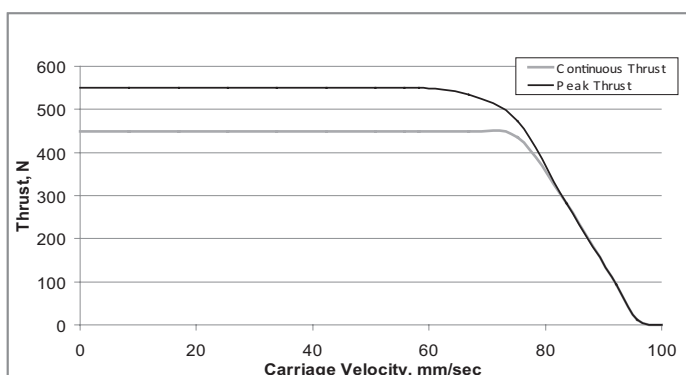
HLD60 Single Rail/Internal Rollers SM23165DT @ 24V, 2.5mm/rev
