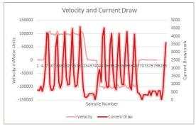
Figure 3: Current draw with velocity overlaid
