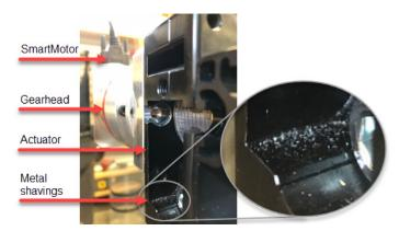
Figure 5: Metal shavings in actuator cavity
