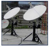
**Big** plans are in M²'s future with the help of the SmartMotor, including a cost-effective means of "auto-tracking." Auto-tracking is accomplished by writing code into the controller unit specifying a certain object's trajectory, while a separate antenna module with receiver is set up to judge signal strength of the object in orbit and automatically adjust the equations in the system to correct the slightest position error and therefore receive the strongest signal data.
