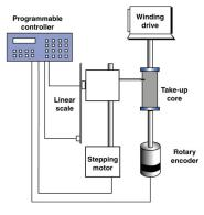
A traditional winding setup with cabling and modules
