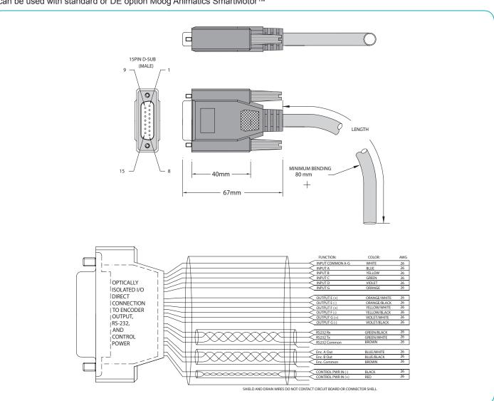
WARNING: Pins 15 and 14 are intended for use with DE series motors for powering the controller only. Attempts to power a non-DE motor through those pins for use as the main servo drive power could result in immediate damage to the electronics and will void the warranty.
