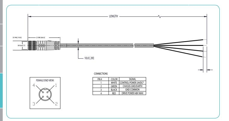
NOTE: Drive Power and Control Power are Separate Inputs. Control power is rated to a maximum range of 18 to 32VDC. Drive Power is from 18 to 48VDC max.
