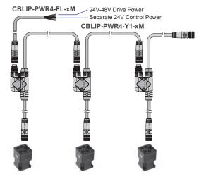
NOTE: Maximum of 15 Amps continuous RMS load per total daisy chain transmission line.
