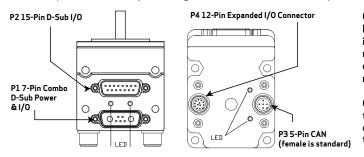
CAUTION: Pins 14 and 15 are intended for use with DE series motors for control power only. Attempting to power a non-DE motor through those pins, as main servo-drive power, may result in immediate damage to the electronics, which will void the warranty.
