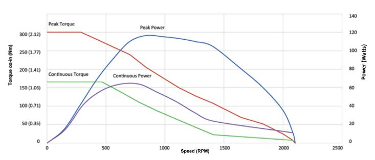
Continuous rating based on 25°C ambient temperature, motor mounted to a 6x6x¼ inch aluminum heat sink, and electronics/windings below maximum temperature. Peak torque is available for 3 seconds at a 10% duty cycle.
