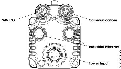
CAUTION: Exceeding 32 VDC into control power on any of the +24V pins may cause immediate damage to the internal electronics. Exceeding a sustained voltage of 48V to pin 4 of the P1 Power Input may cause immediate damage to the internal electronics. Exceeding these voltage limits will void the warranty.
